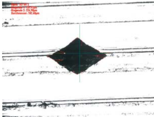
Fig. 2. Surface of the test rings. It is easy to see the dark area of identification, the black lines are grooves caused by the lathing operation. The measured hardness is 165HV
