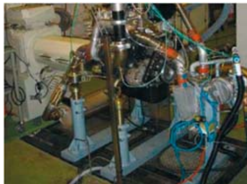
Fig. 4. IVECO engine F1C with the dynamic dynamometer
