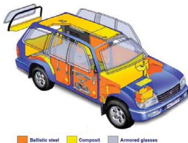
Fig. 13. The example of elements of the protection fastened inside the vehicle [4]
