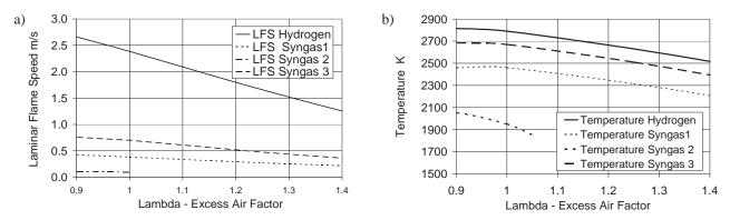
Fig. 1. Laminar flame speed (LFS) (a) and adiabatic temperature (b) vs excess air lambda for various mixtures of gaseous fuels and air at NTP conditions 25°C, 101,325 Pa
