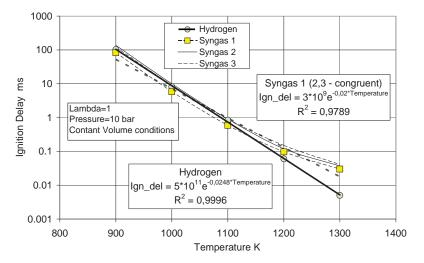
Fig. 2. Ignition delay vs temperature for hydrogen and various syngases at stoichiometric ratio with air
