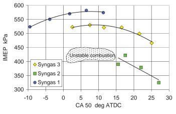
Fig. 10. IMEP vs CA50 for syngases 1, 2 and 3
