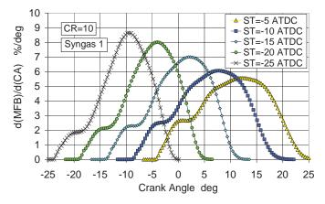
Fig. 6. MFB rate of combusting syngas 1 with various spark timings
