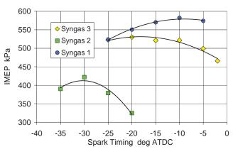
Fig. 4. IMEP vs spark timing for combustion tests of syngases 1, 2 and 3
