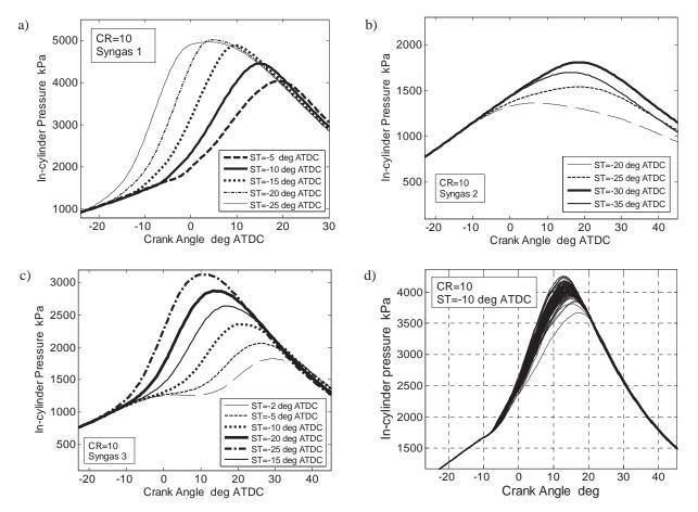
*Fig. 3.* In-cylinder combustion pressure histories for: *a*) syngas 1, *b*) syngas 2), *c*) syngas 3; at various spark timings, *d*) Set of 100 in-cylinder pressure traces for syngas 1
