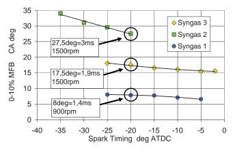
Fig. 8. 0-10% MFB vs spark timing for syngases 1, 2 and 3
