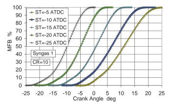
Fig. 5. MFB profile of combusting syngas 1 with various spark timings
