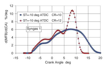
Fig. 7. MFB rate of syngas 1 combustion at compression ratio of 10 and 12
