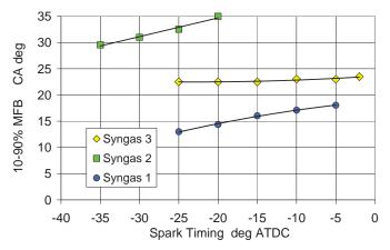
Fig. 9. 10-90% MFB vs spark timing for syngases 1, 2 and 3
