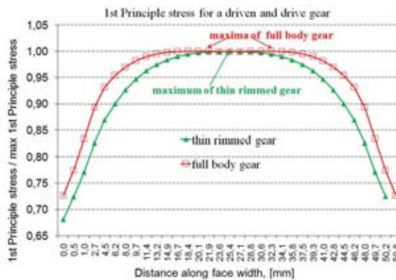
Fig. 3. Comparison of 1st principle stress layout between full body and thin rimmed gear
