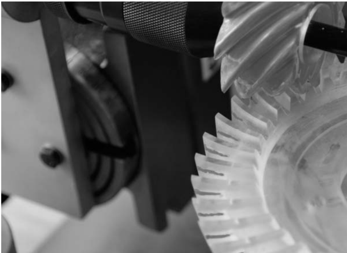
Fig. 6. Contact area of test hypoid gear transmission
