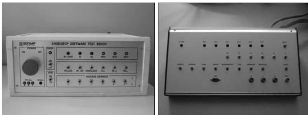
Fig. 4. Exemplary research tools used to optimise software of the integrated avionics system: the SHUD/UFCP tester (left), and the Multi-function Display (MFD) tester (right)
