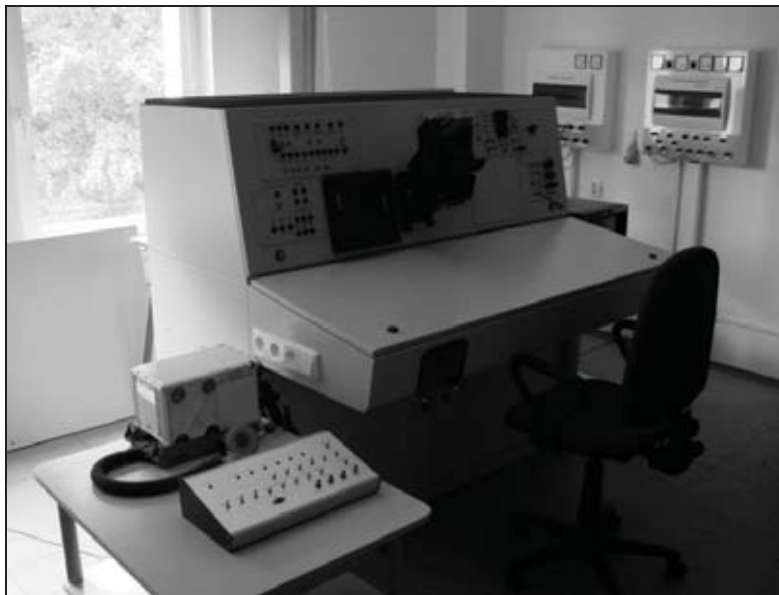
Fig. 2. The laboratory equipment to optimise integrated avionics systems on the digital data bus MIL-STD-1553B
