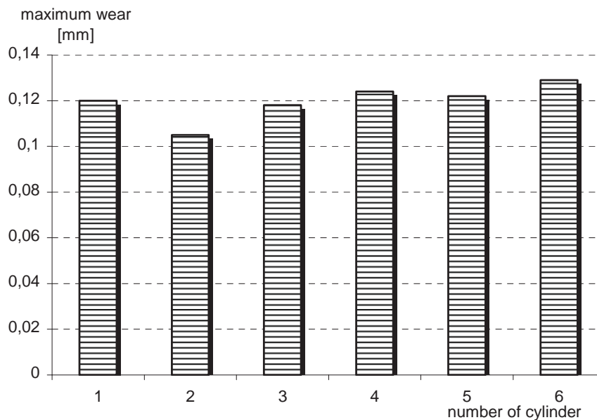
Fig. 2. Maximum wear and tear of cylinder liners of a 359 engine after a mileage of 204864 km
