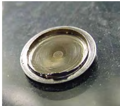
Fig. 7. The Oprtrand pressure sensor membrane damage
