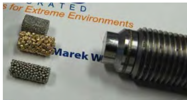
Fig. 8. The flame suppressors to the Oprtrand pressure sensors
