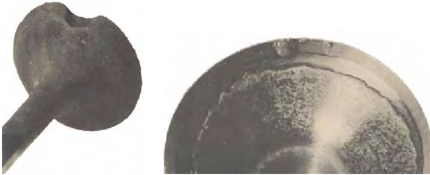
Fig. 10. Example valve damage resulting from the presence of carbon deposit
