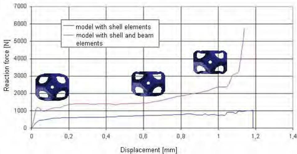
Fig. 10. The comparison of the reaction force – displacement charts for two numerical models of the open cell foam microstructures (made of shell and beam and shell elements) resulted from the FE analysis
