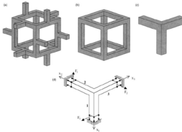
Fig. 3. Unit cell geometry and boundary conditions: (a) open structure; (b) simplified; (c) one-eighth; (d) under triaxial loads [5]
