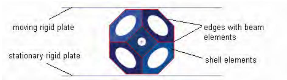
Fig. 6. The numerical model – finite elements and boundary conditions
