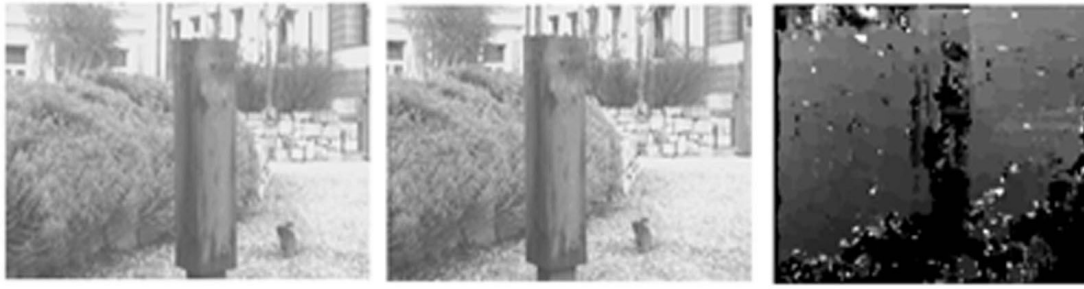
Figure 2. Image motion field of right camera: a) Image at t_{i-1} ; b) Image at t_i ; c) Image motion field.
