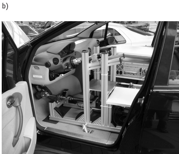
Figure 3 a) The Mechanical design of the driving robot, b) Integration of the robot in the car
