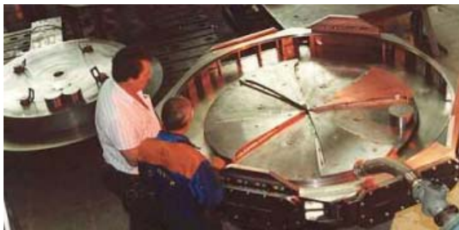
Fig. 3. In foreground – bottom pole with vacuum chamber, on the left – top pole with cover of vacuum chamber.
