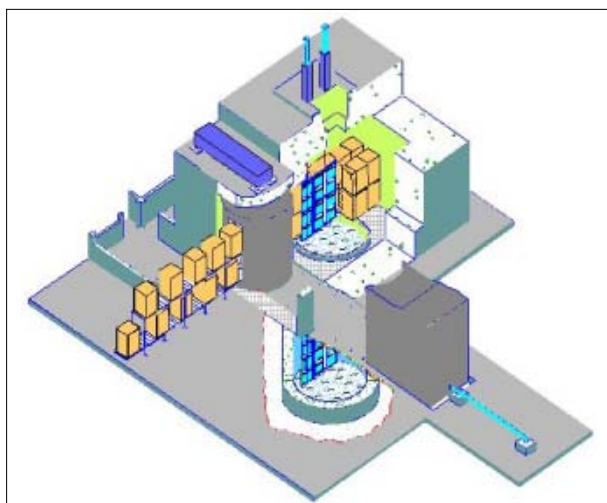
Fig. 1. Scheme of rotating door irradiator [19].
