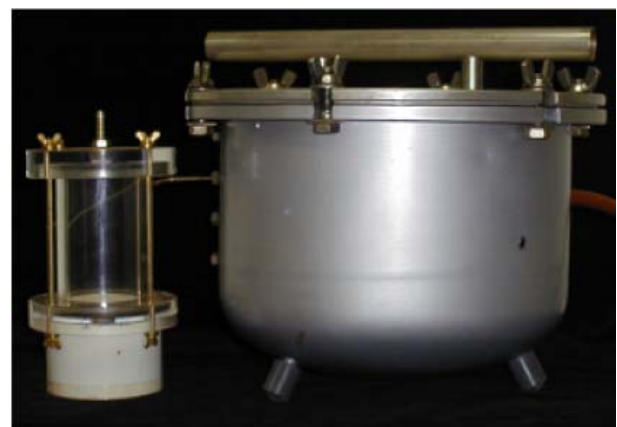
Fig. 3. Side view of the projected pressure chamber and the commercial low-pressure chamber.
