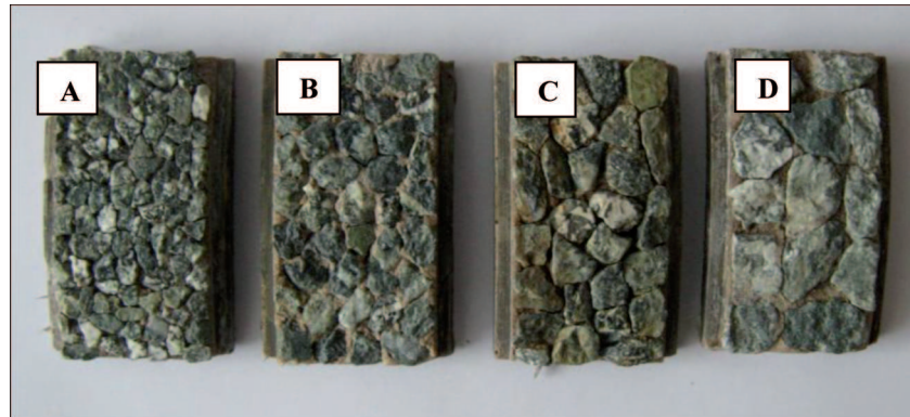
Fig. 2. Specimens of gabbro aggregate for test into resistance to polishing according to the British method (aggregate size: A – 4/6.3, B – 8/10 – standard specimen, C – 10/12.8, D – 12.8/16).
