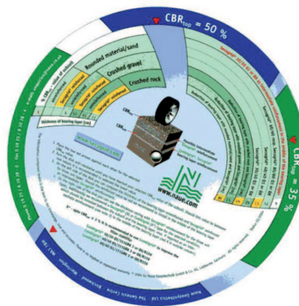
Fig. 17. Design disc for bearing layer reinforcement in traffic areas using welded Secugrid ® geogrids.
