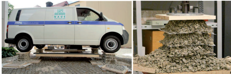
Fig. 7. Geogrid reinforced gravel columns carrying a van (left) and pretesting of gravel columns in the lab (right).
