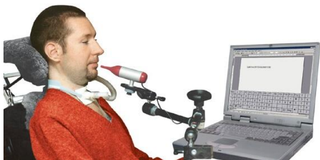
Rys. 6. System sterowania ustami Integra Mouse [7] Fig. 6. Integra Mouse control system operated with mouth [7]
