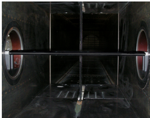
Fig. 3. ILH412 airfoil in N-3 wind tunnel
