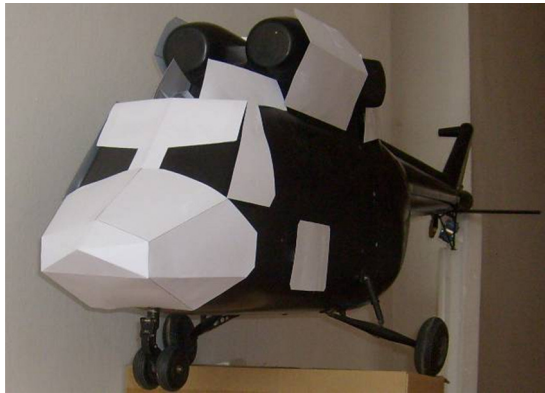
Figure 1. Armour concept for 6-ton take-off weight multipurpose helicopter
