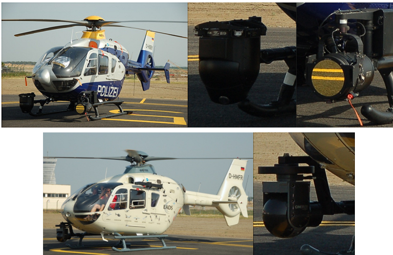
Figure 1 Examples of external components on the modern helicopters (camera) (c) Adam Dziubiński
