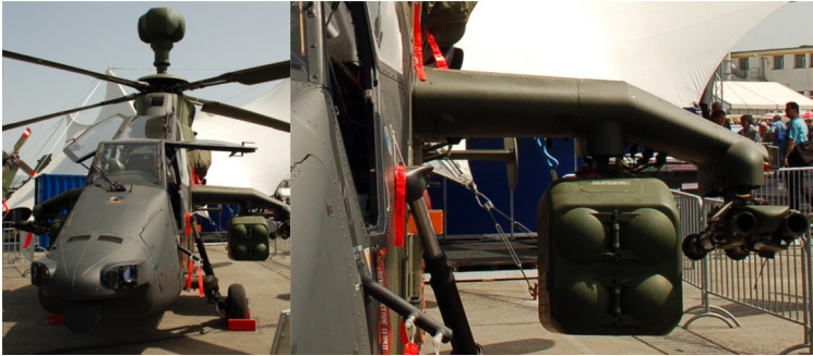
Figure 3 Example of external components on the modern helicopters (wings, pylons, tanks) (c) Adam Dziubiński
