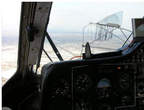
Figure 2. A special indicator mounted in front of the windshield used to maintain near-zero velocity relative to the ambient air
