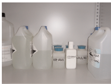
Fig. 2. Row solutions (low concentration), samples of HTP (87,6%) and concentrated (stabilized, 86%) H 2 O 2 prepared with the use of special vacuum rotary evaporator by the authors
