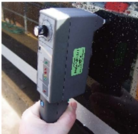
Rys. 7. Tap test – (Wavelength NDT [3])
