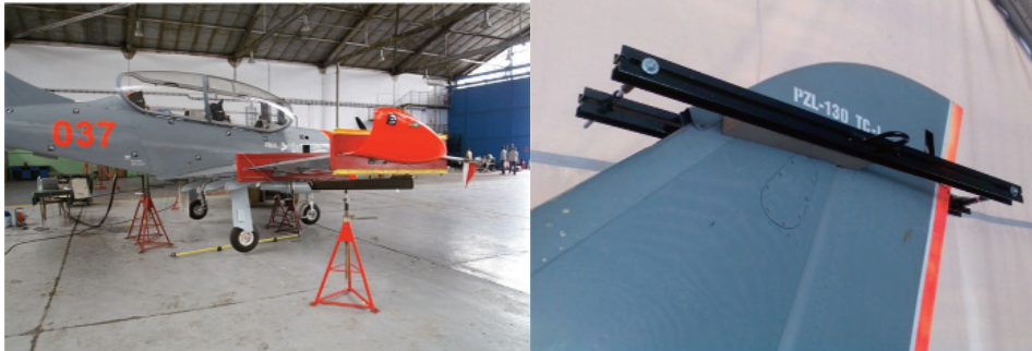
Wing sensors calibration and clamps used for wing and fin loading
