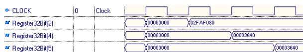
Rys. 5. Cykl pracy sterownika PLC w FPGA Fig. 5. The cycle of the work of the controller in FPGA
