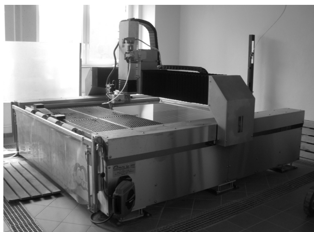
Fig. 5. CNC WJ2020B-1Z-D device from PTV company used for preparation of the samples by AWJ technology
