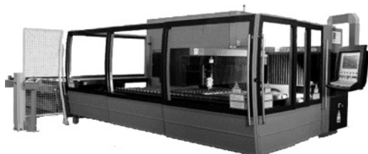
Fig. 6. 2D CNC PLATINO 2040 /3500 CP device used for preparation of the samples by CO 2 laser cutting technology [6]
