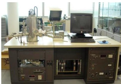
Fig. 1. The PHI model 4200 set-up used for AES measurements
