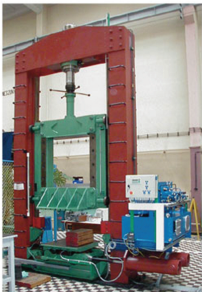
Fig. 11. 40 T press for L/G static tests (picture:IA archive)
