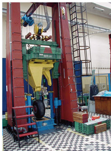
Fig. 12. 10 T drop machine for L/G dynamic tests (picture IA: archive)
