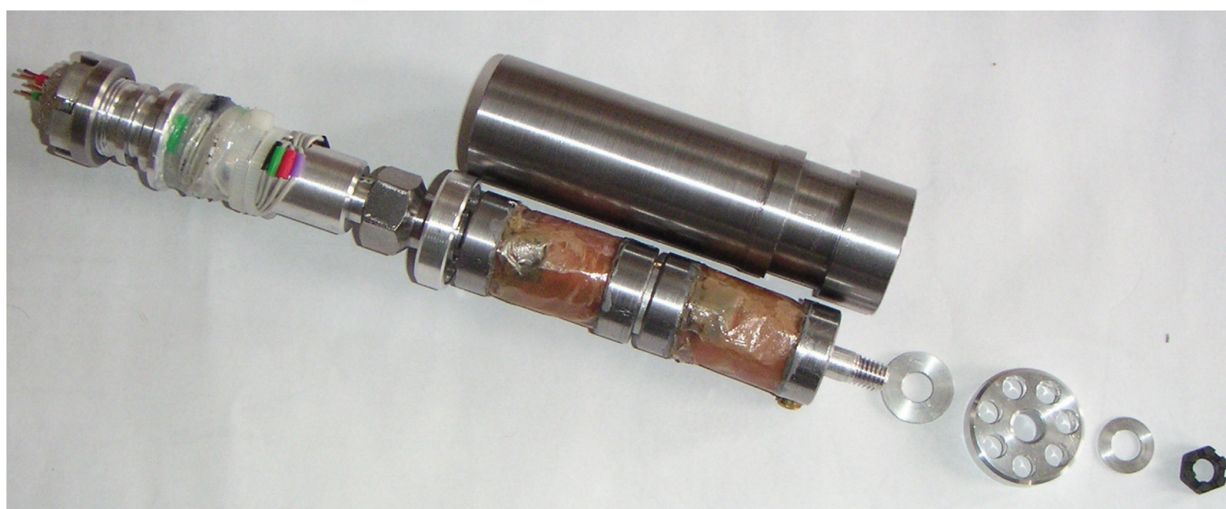
Fig. 10 Prototype of MRF based shock absorber – internal parts
