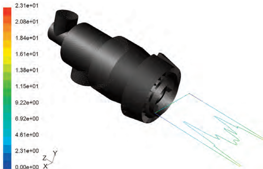
Figure 4. Geometry of the numerical model of the burner and the profile of velocity magnitude [m/s] at a distance of 20 cm from the outlet
