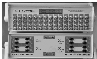
Rys. 3. System RLC i zestaw wzorców C i R Fig. 3. RLC system and a set of the C and R standards
