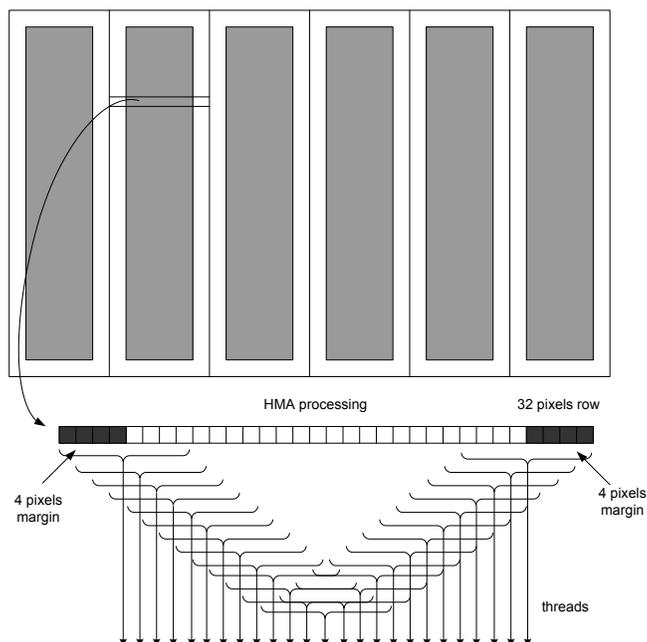
Fig. 2. The idea of the HMA processing
