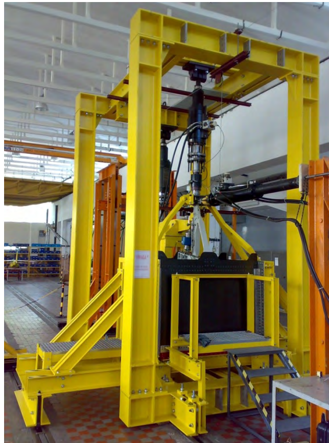
Fig. 3. Test set-up with the A400M VTP actuator hinge fitting specimen.
