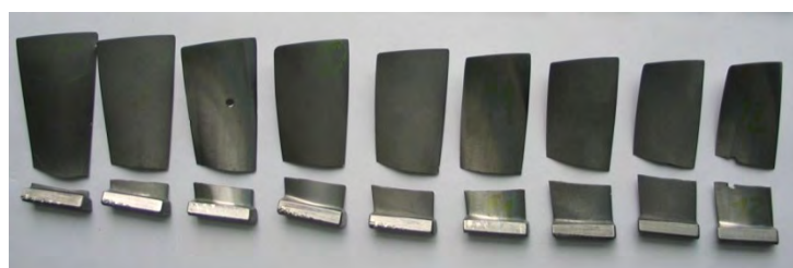
Fig. 8. Ruptured blades of the 1-st stage of the compressor after investigations.
