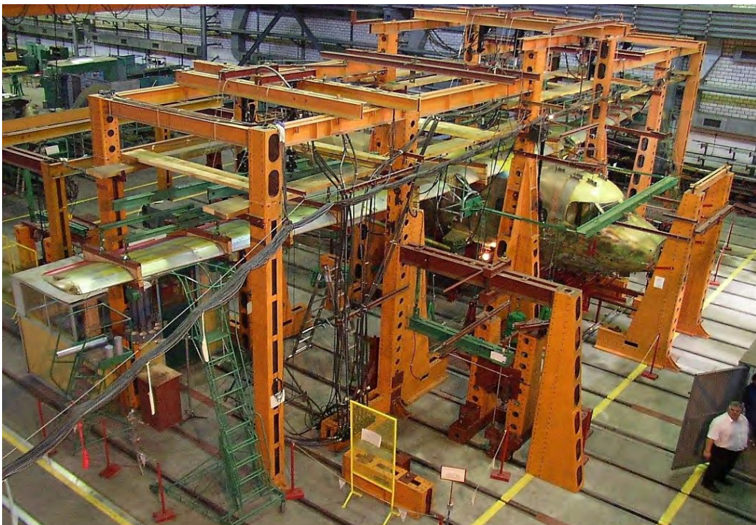
Fig. 2. Wing and wing loads-carry-through test rig. The test is conducted with MTS Aero 90-LT system.
