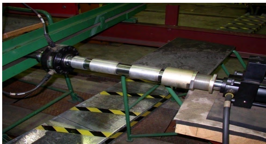
Fig. 6. MTS Aero 90-LT hydraulic actuator with stroke limiter, used in order to prevent extensive damage of tested airframe in case of the loss of its rigidity.
