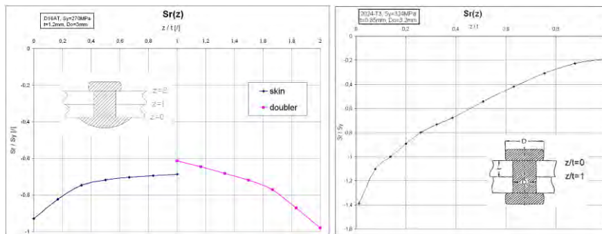
Fig. 5. Residual radial stresses through the thickness on the edge of the hole; left) at present work, right) based on PhD thesis of Mr. Muller
