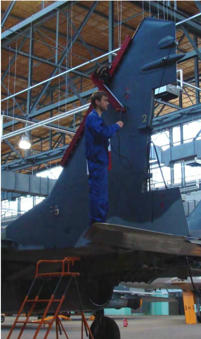
Pic. 1. Composite vertical stabilizer inspection.
