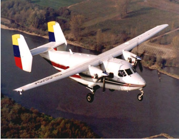
Fig. 1. PZL M28 05 "SKYTRUCK" aircraft in flight. Twin turboprop, braced wing, fixed landing gear light transport airplane. Unpressurized fuselage. Strut-braced wing. Twin-fin tail.
