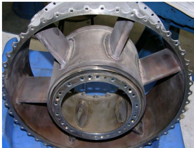
Fig 1. View of a turbine casing for the small helicopter turbo-engine.
