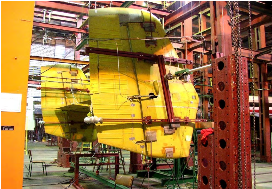
Fig. 3. Empennage test rig in Polskie Zaklady Lotnicze. The test program was prepared by the Institute of Aviation in Warsaw. The loading system was developed at PZL Mielec.
