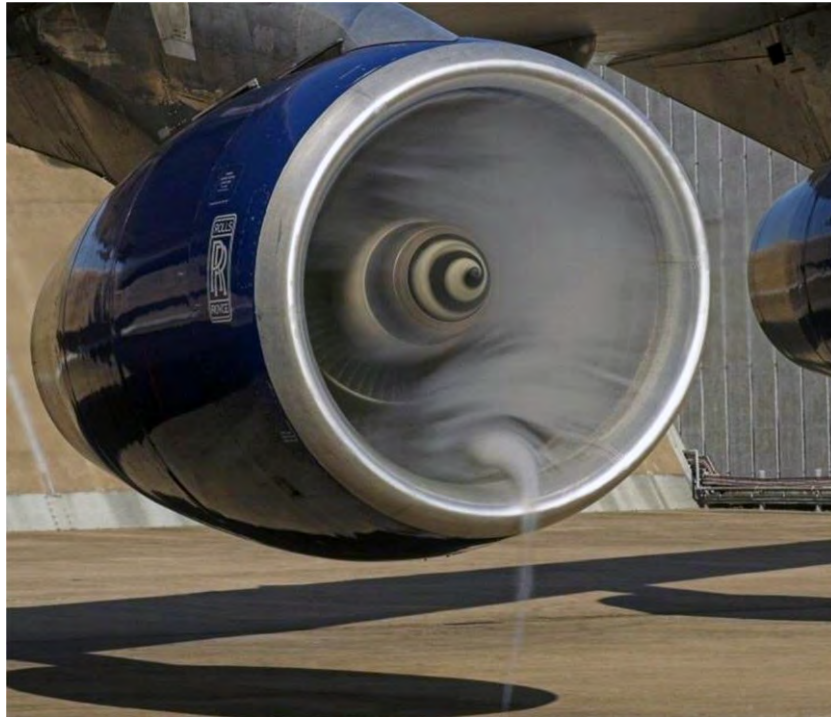
Fig. 5. Photo of inlet vortex, taken during engine ground test (Rolls Royce Trent 560 engine on Airbus 340-600 airplane)
