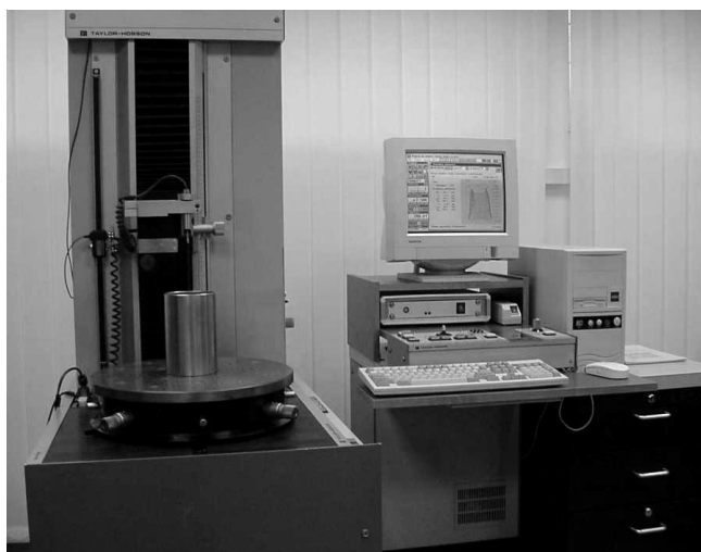
Fig. 3. Taylor-Hobson Talycenta incorporated in the developed computer-based measurement system.
