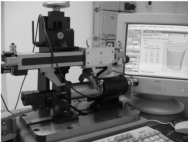
Fig. 1. The model measuring device PSA 6 for the measurements of cylindricity profiles with the reference method
