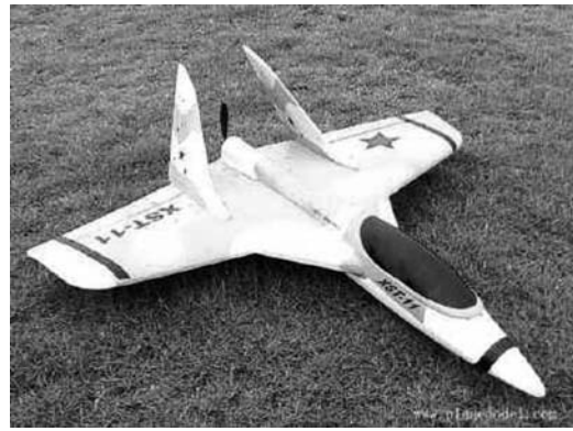
Fig. 6. Expanded Polystyrene (EPP) airframe
