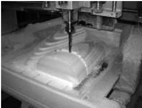
Fig. 2. CNC milling of 3D fuselage male mould of a small UAV
