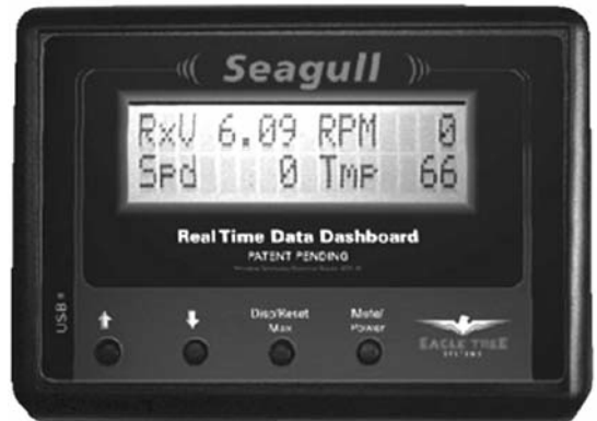
Fig. 18. The Eagle Three telemetry link terminal [12]
