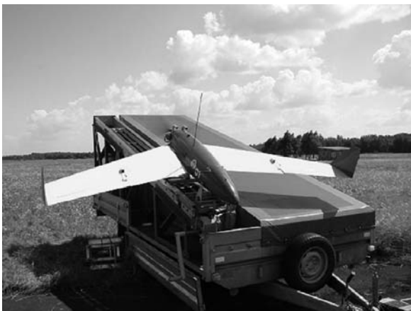
Fig. 8. Small UAV takes off from the rubber launcher
