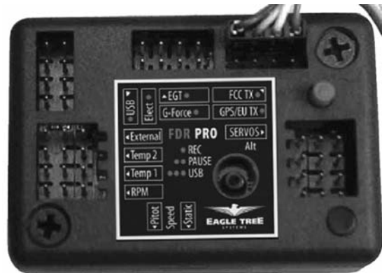
Fig. 17. The Eagle Three - the onboard flight data acquisition unit [12]
