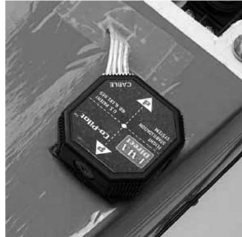
Fig. 12. Co-pilot sensor head [11]
