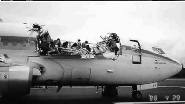
Structural failure of an Aloha Airlines Boeing 737 on April 28th, 1988 [5], by effect of small fatigue cracks extending from adjacent rivet holes in a fuselage lap-splice joint
