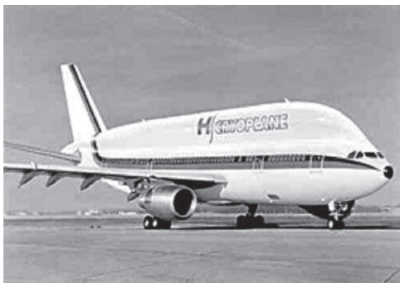
Fig. 6. The studio project of A - 320 airplane in case of engines fueling by the liquid hydrogen (extremely big fuel tank in fuselage)
