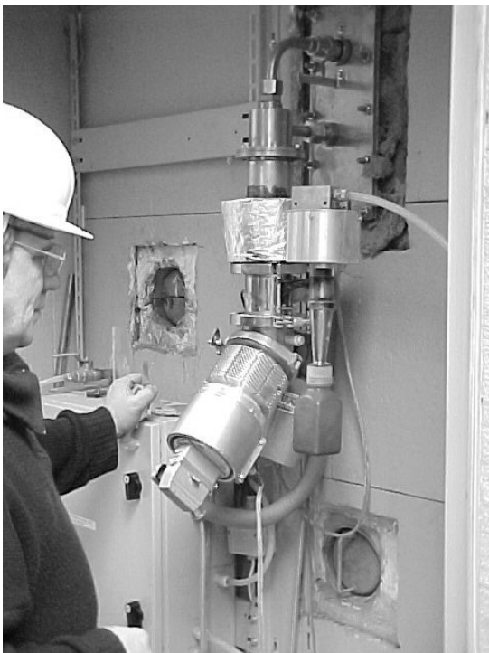
Rys. 7. Głowica pomiarowa na kanale emisji spalin w elektrowni Fig. 7. Optical measurement head mounted in the power plant emission channel
