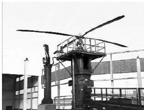
Fig. 4.27. Eurocopter BK-117 smart rotor in test stand
