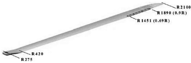
Fig. 4.25. The Rotor r Pales Actives (RPA) blade with flaps actuated by APA
