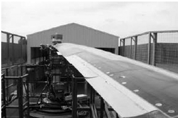
Fig. 4.29. Rotor blade with trailing edge flap actuated with magnetostrictive actuators and extension-torsion coupled composite tube
