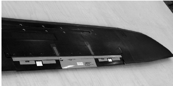
Fig. 4.25. The Rotor r Pales Actives (RPA) blade with flaps actuated by APA
