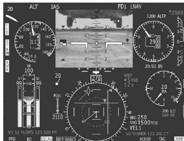
Fig. 2. UH-60M PFD Modified with FLIR Landing Zone Video
