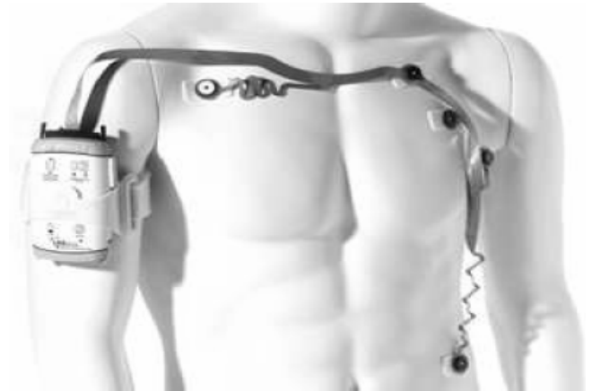
Fig. 2. LifeSync® Wireless ECG – ECG and respirometry system; patient module [10]
