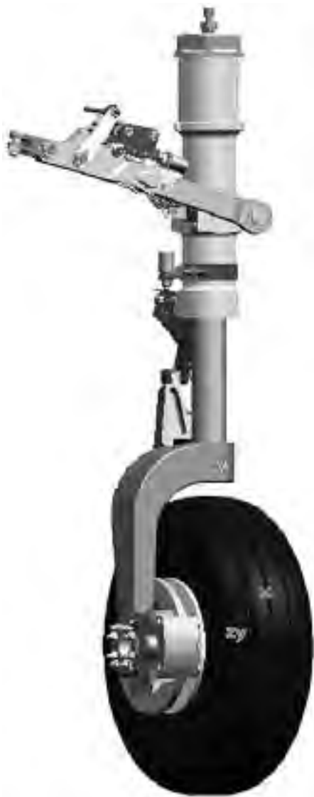
Fig. 16. Main retractable cantilever type landing gear for light aircraft – 3D model
