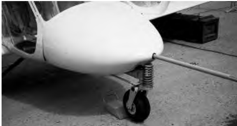
Fig. 20. Non-retractable landing gear landing gear with steel ring spring
