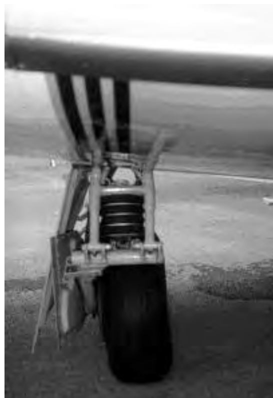
Fig. 19. Retractable landing gear with spring rubber elements
