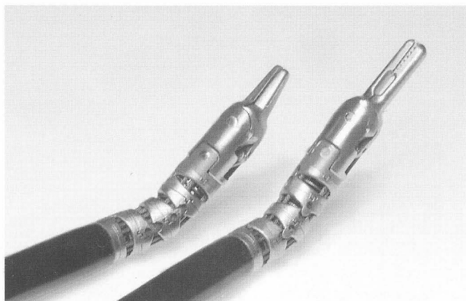
Fig. 2. Robotic gripper da Vinci (Intuitive Surgical) with increased degrees of freedom driven by the system of wires and less diameter.
