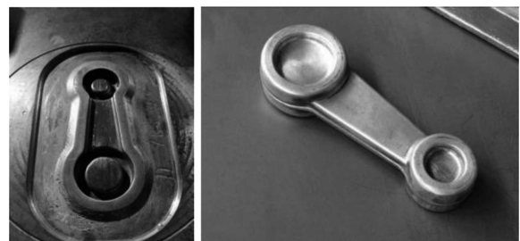
Fig. 4. Die insert to forge a model of connecting rod and model of connecting rod forged from magnesium alloy
