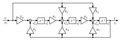
Figure 1. State variable diagram for (28).
