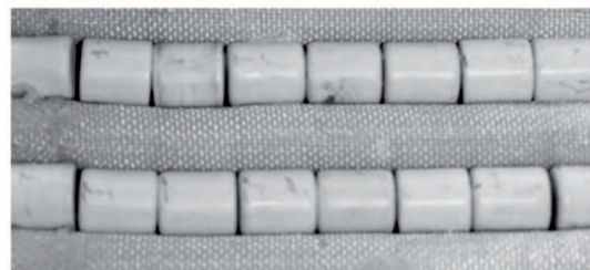
Fig. 4. Scheme of separation of ceramic components (1) by means of a flexible interlayer (2)
