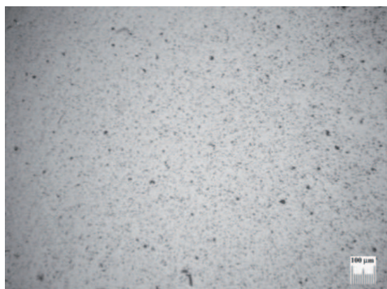
Fig. 4. The image of sintered sample made of paste with Ferro resin from the light microscope (magnification x100)
